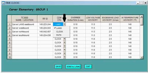
between the LANG and clock via a chain of one or more clocks. The PATH function is selected by clicking on the arrow on the right of the COM CFG column. Selecting PATH will open the 'RF ROUTING' window. The RF ID for each clock in the path is entered, starting with the clock closest to the LANG and ending with the one closest to the pathed clock. Click 'DONE' to save the path information (Figure 3.4.5).
