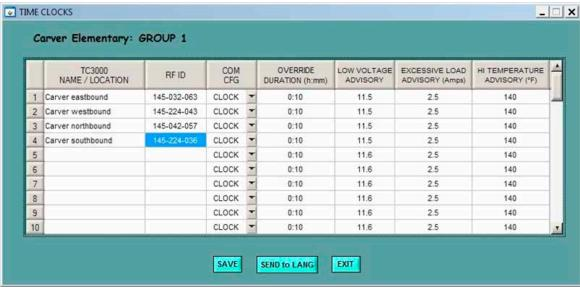
The COM CFG field is used to define the unit as a LANG or clock and to define the path for repeater functionality (Figure 3.4.4). The LANG can be used as a clock, but must be the first clock in the first group. **Repeater** functionality is available when a clock cannot be reached directly by the LANG. A path is established
